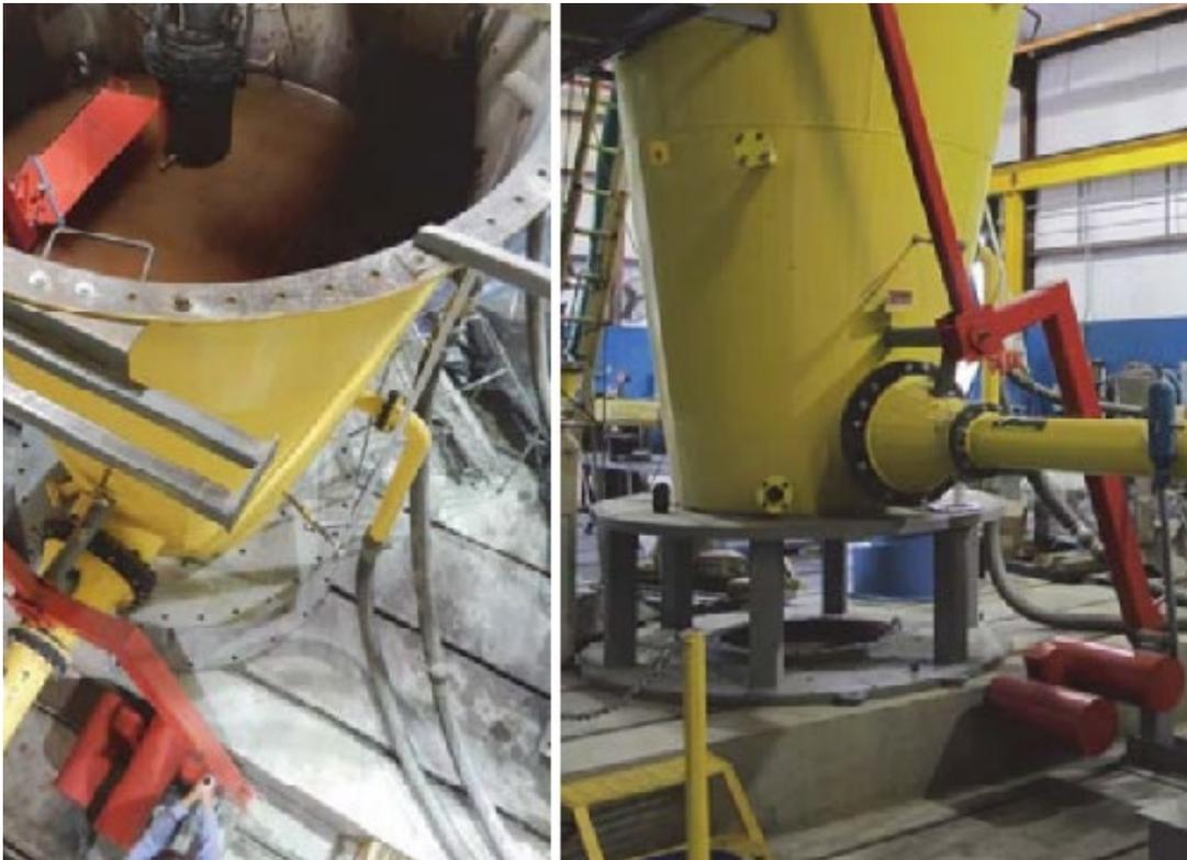
The research team developed a remarkably comprehensive loop test program. Their tests, which consisted of very carefully sourced components, featured a large, 203-mm diameter pipe loop and tank filled with thousands of liters of water. Researchers used an excavator to deposit various solids into the tank. Once they added the appropriate tonnage, they gradually increased the pipe velocity up to 7 meters per second, causing the particles to flow through the system.
